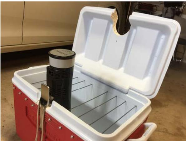
Cap nuts (8-32) secure the protruding ends of the rods; they are anchored with Liquid Nail adhesive rather than threads.
