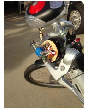
This photo shows the device with the cap removed. There are only nine electronic parts which includes a FET and an LM555 timer chip. Charger owners who would like free detailed specs can click on Visitor Comments and submit a request.
