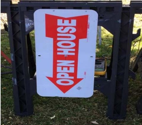
This experiment is the same as experiment #1 except that the earth surface is turf rather than concrete. The plate/earth Configuration is a vertically oriented 24" x 12" metal plate elevated so its center is 19" above the earth surface.
