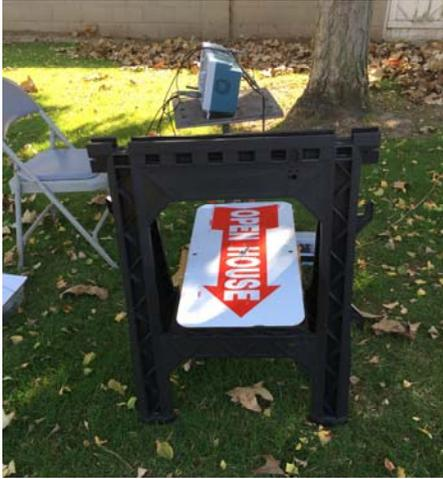
This experiment is the same as experiment #2 except that the plate is oriented horizontally instead of vertically. The plate/earth Configuration is a horizontally oriented 24" x 12" metal plate elevated so its center is 19" above the earth surface.
