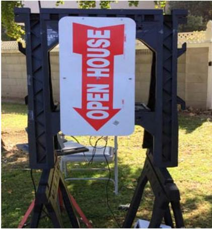
This experiment is the same as experiment #2 except that the plate is at a greater height. The plate/earth Configuration is a vertically oriented 24" x 12" metal plate elevated so its center is 50" above the earth surface.
