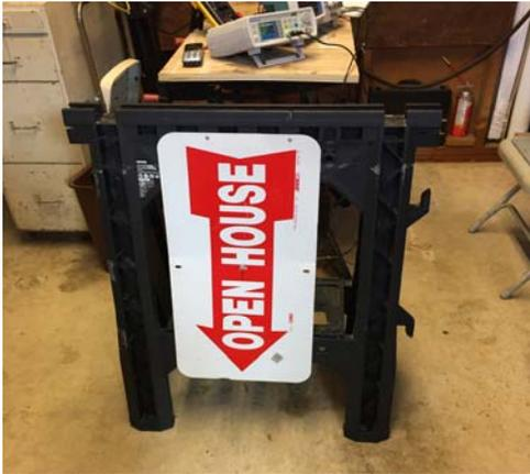
The plate/earth Configuration is a vertically oriented 24" x 12" metal plate elevated so its center is 19" above the earth surface. The earth's surface is concrete with imbedded rebar.
